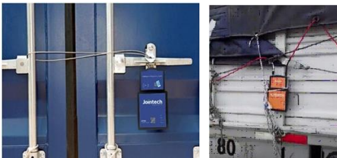
Figure 3-40: Examples of Cargo Seals with ECTS
