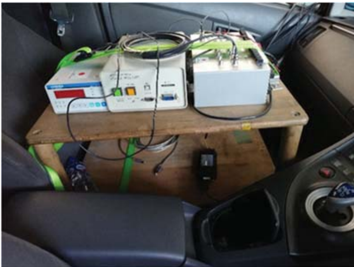
Example of measurement vehicle for impact of reducing exhaust gas before and after the introduction of the eco-driving
