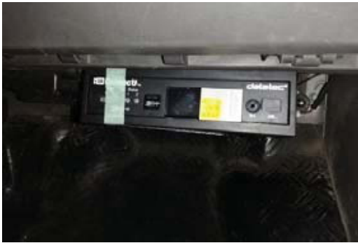
The eco-driving support device installation example
