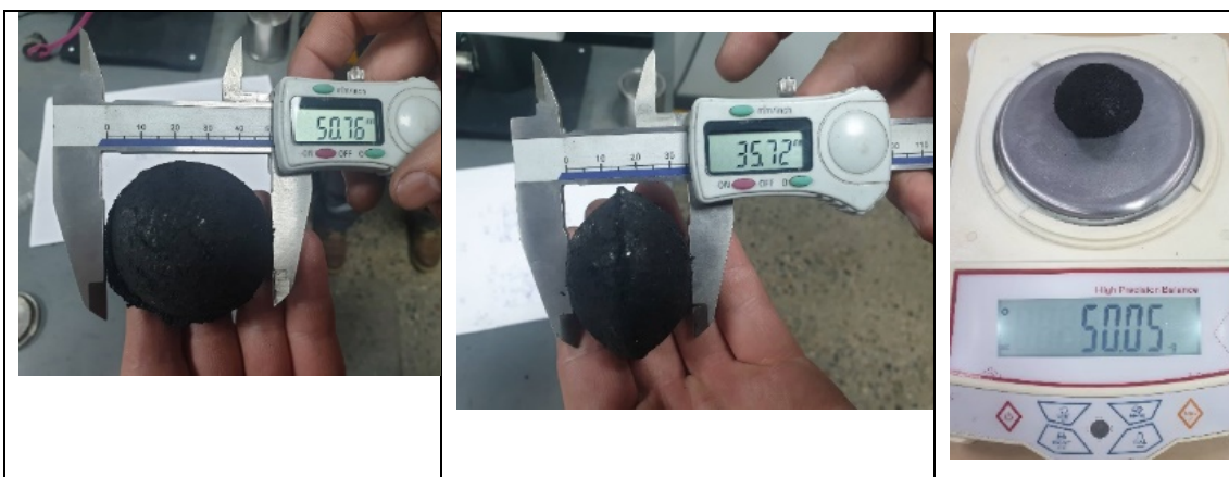
30. Pilot plant biomass briquette size 50.76mm x 35.72mm. 1 pcs weight without dried = 50.05 gr
