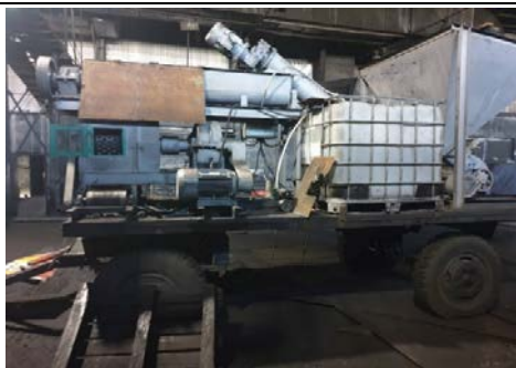
24. Mobile pilot plant which planning to do test in power plant 2
