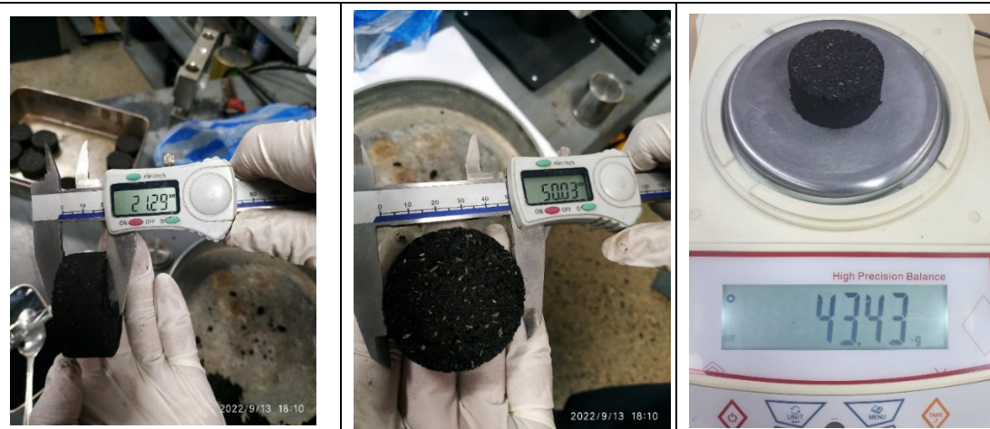
23. Tablet test 21.29mm x 50.03 mm, after dried weight 43.43 g
