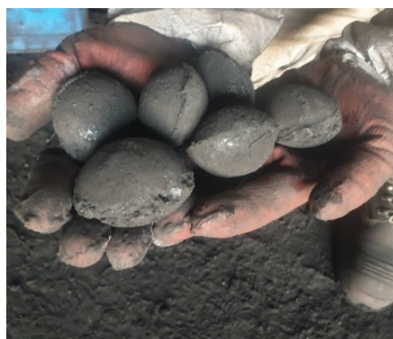
26. Biomass briquette: Sawdust 10%, Mongolian binder 6%, water 15%
