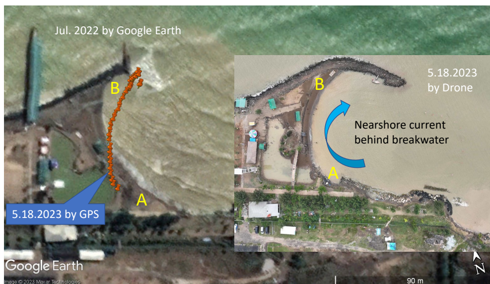
Figure 71 Mechanism of topography change in the survey point No.2
