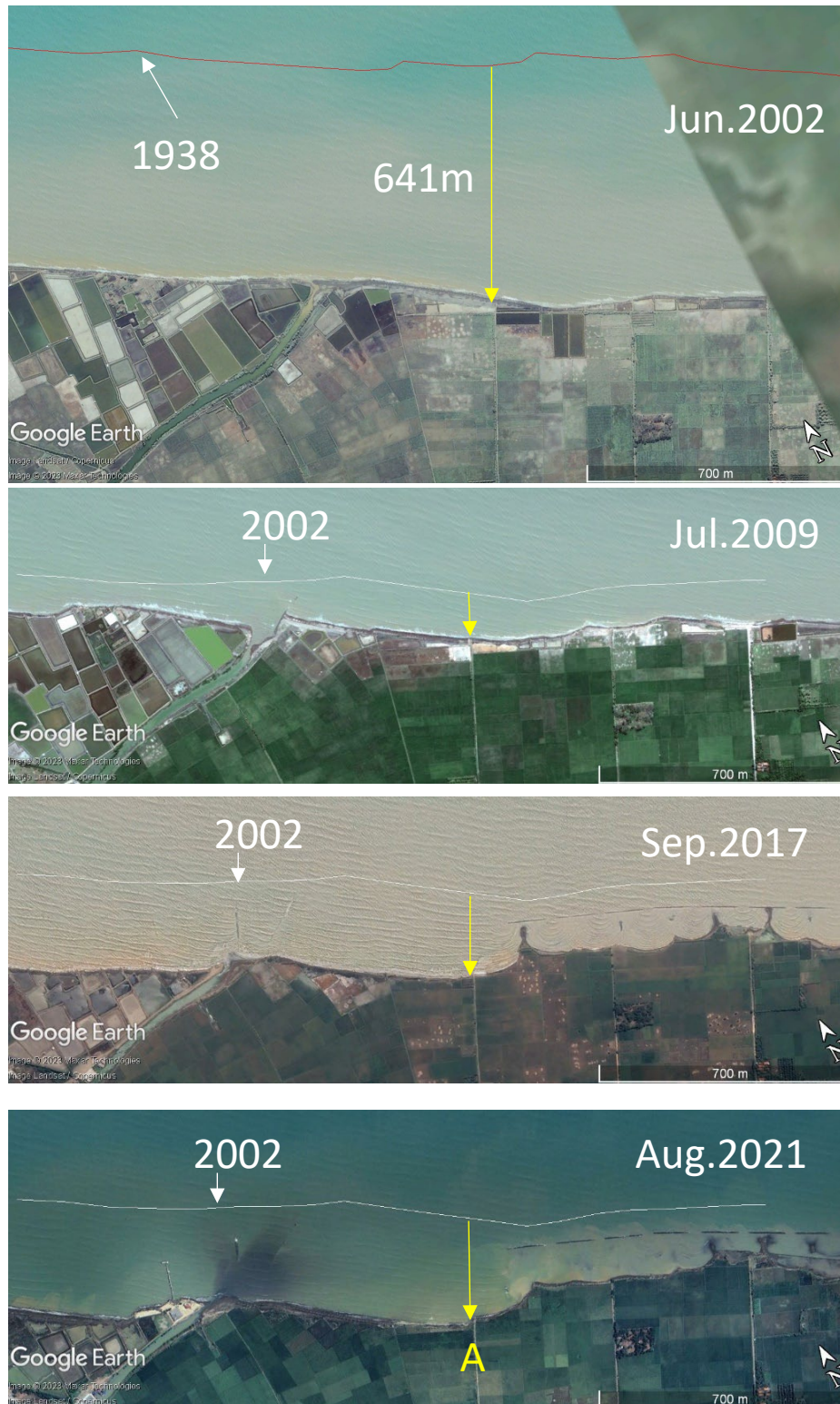
Figure 38 Topographic change around offshore breakwaters in Indramayu East
