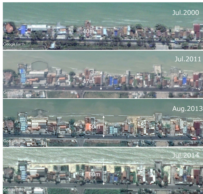
Figure 86 Topography change around offshore breakwaters in northern side of reclaimed land(Point A)
