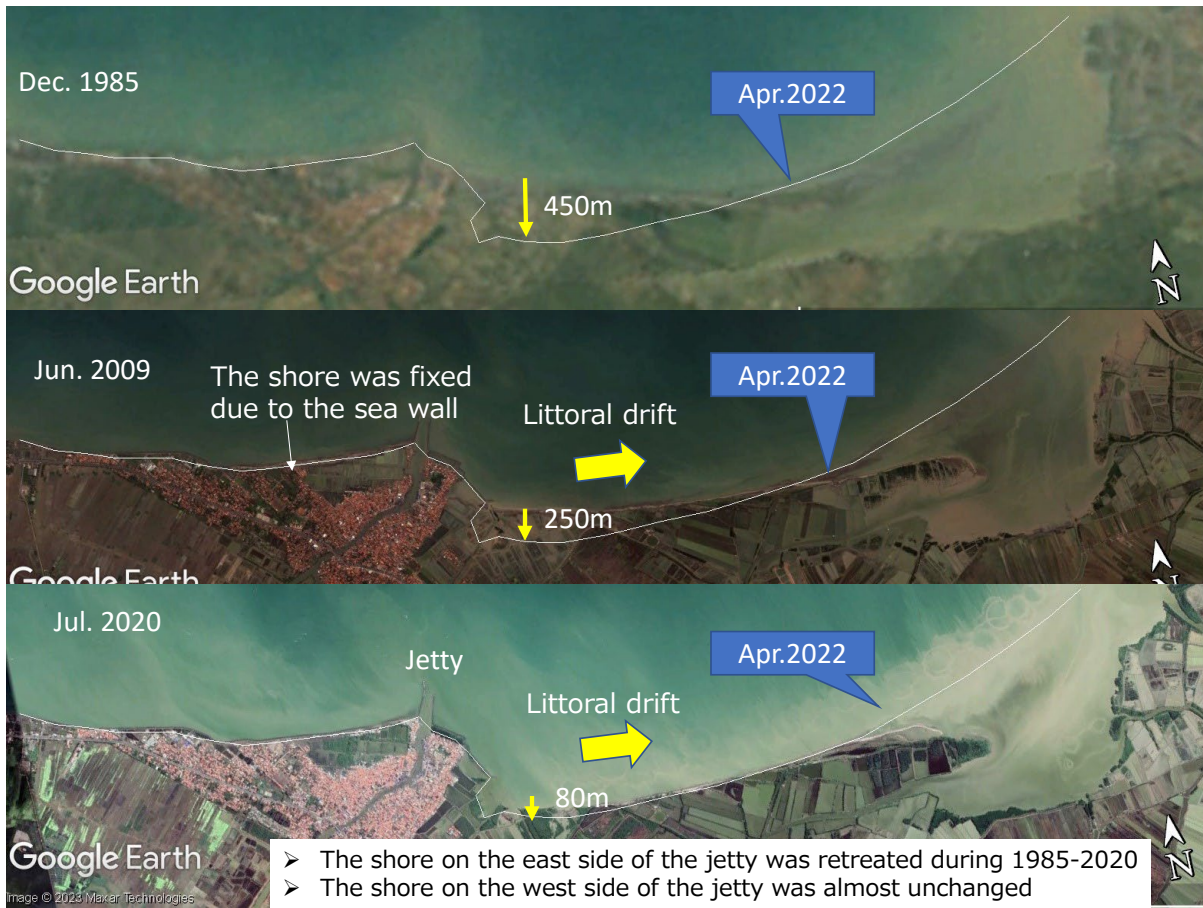
Figure 77 Topography change process of the step A in Indramayu West
