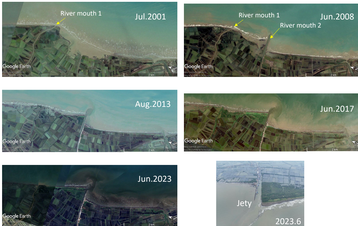
Figure 80 Topography change process due to the construction of jety at the step B in Indramayu East
