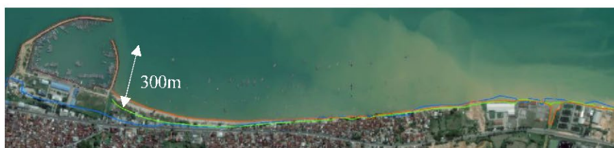
Figure 103 Shoreline Change Caused by Trapping Longshore Sediment Transport
