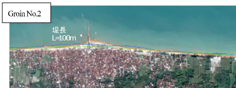
Figure 102 Shoreline Change Caused by Trapping Longshore Sediment Transport
