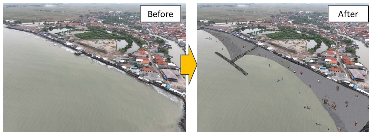
Figure 4.2 Image of Before- and After-Implementation of Beach Nourishment and Headlands (Area-I, S-1a)
