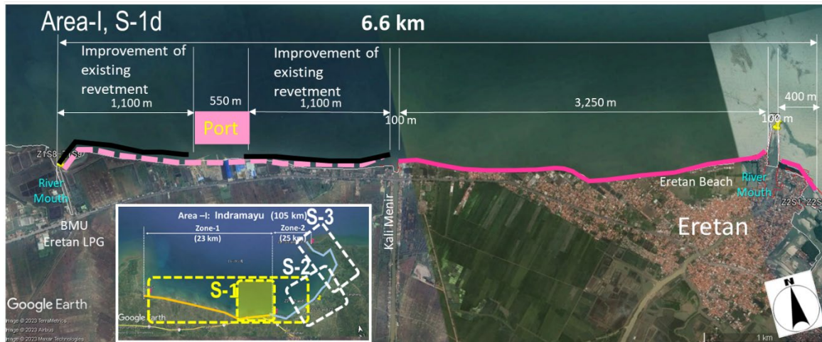
Figure 13.5.5 Coastal Facility Plan at Indramayu Section-1d
