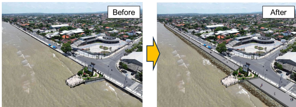
Figure 13.3.14 Image of Before-and After-Implementation of Type-1 Revetment in Tuban (T-b)
