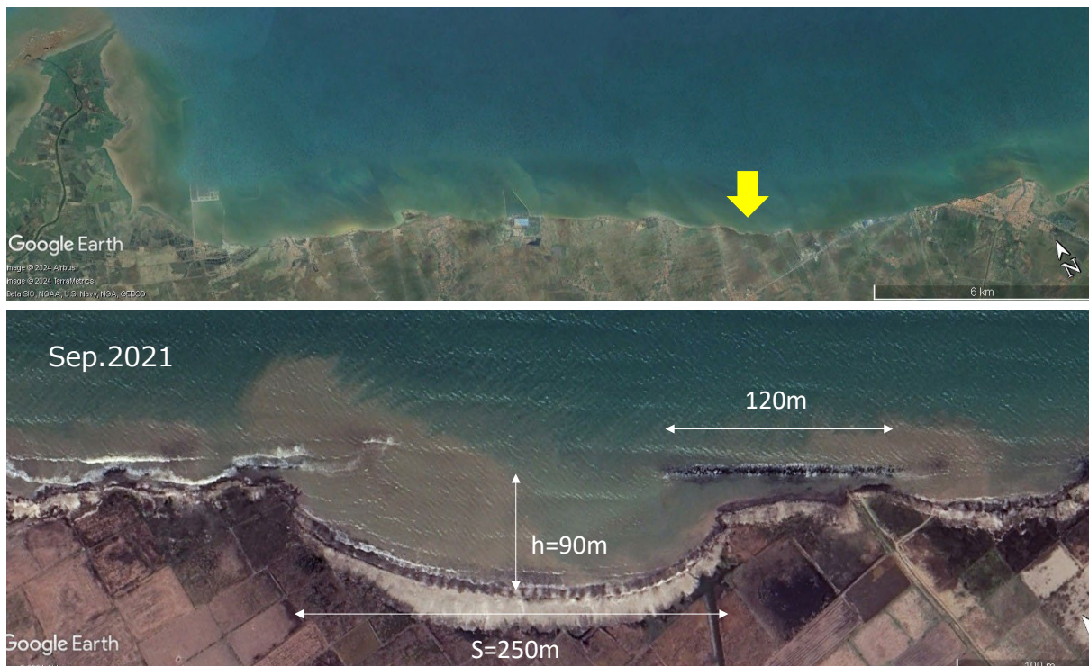
Figure 13.4.2 Example of Stable Curvature Topography (Indramayu)
