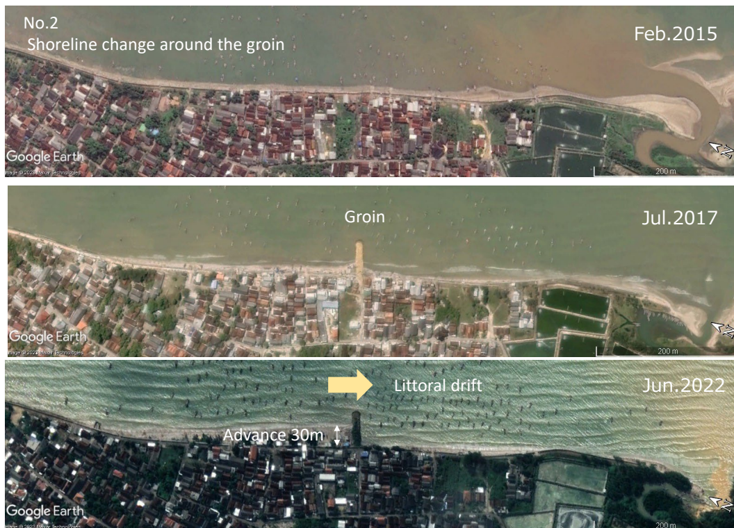
Figure 12.2.8 Shoreline Change Around the Groin (No.2)
