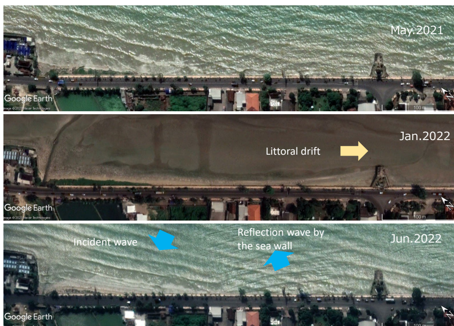
Figure 12.2.12 Shoreline Change Around the Reclaimed Land and the Groin (No.4-b)
