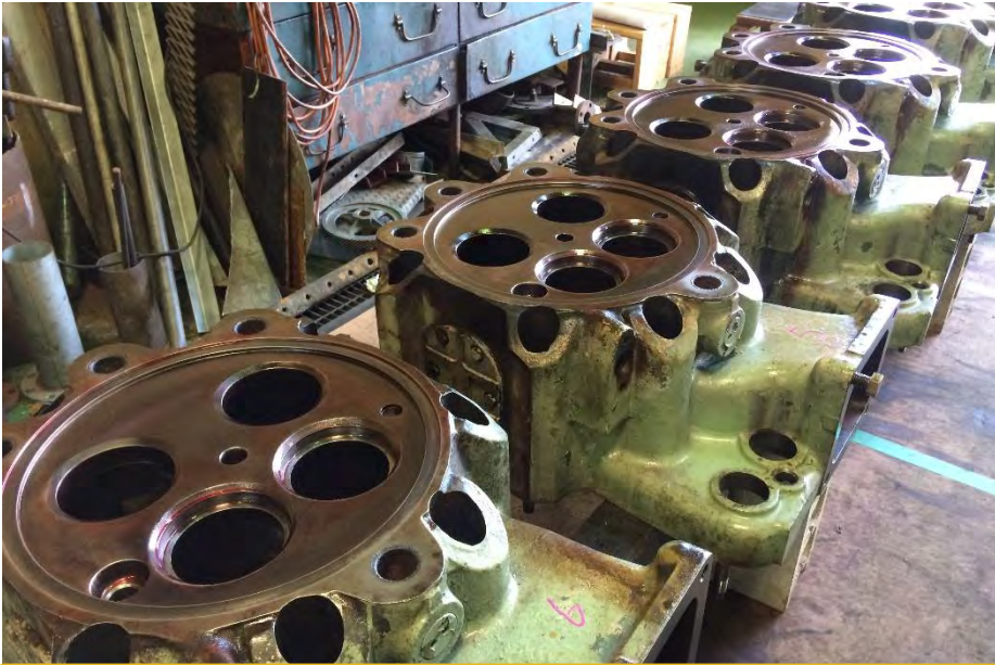
Cylinder Head color check
