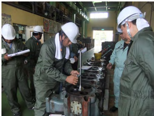
Engine part measurement, dye penetrant test
