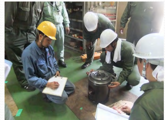
Engine part measurement, dye penetrant test
