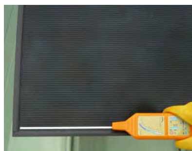
<Busbar detection for compound semiconductor module>
