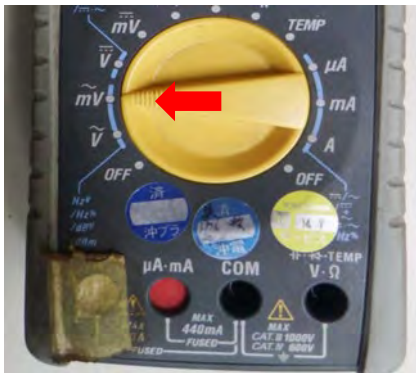
Voltage range (thermocouple inspection)
