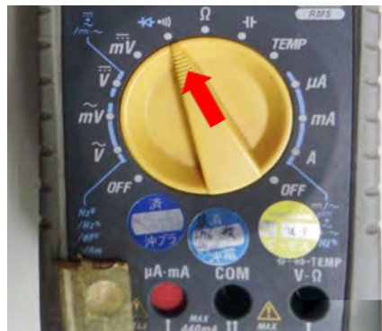
Buzzer (Pressure switch test)
