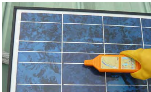
<Interconnector detection for c-Si modules>
