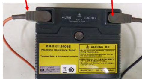
Connect the lead wires to the connector on the back of the megger
