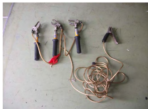
Short-circuit ground wire
