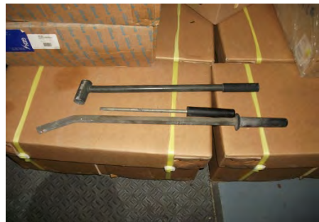
Circuit breaker handle
