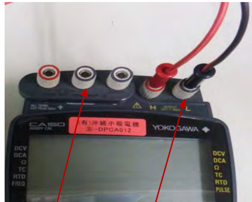
OUTPUT terminal INPUT terminal The opposite side (clip side) of the lead wire is connected to the measuring instrument
