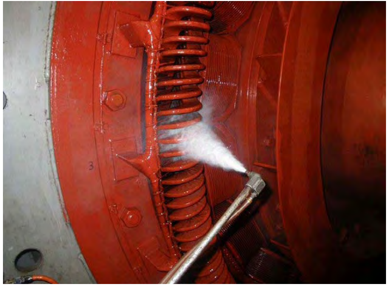
▪ Washing with an electrical cleaning agent
