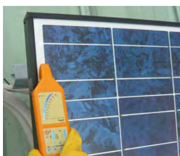
<Busbar detection for c-Si module>
