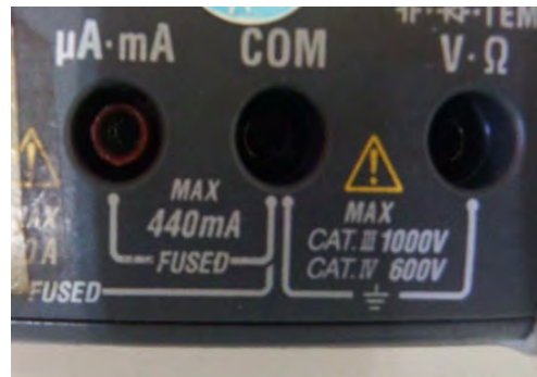
In case of current measurement, mA · COM For voltage and resistance measurement, V · Ω and COM
