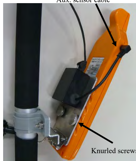
&lt;Receiver mounting (rear side)&gt;
