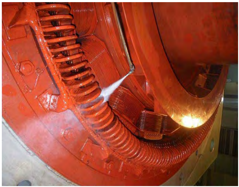
▪ Washing with an electrical cleaning agent
