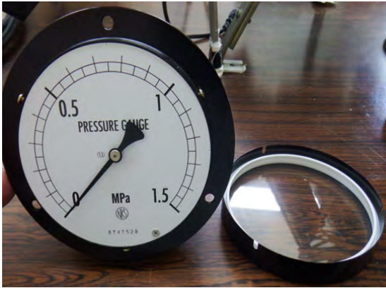
Loosen the cover mounting screws (3 places)
