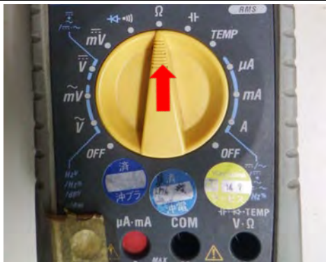
Resistance range (continuity test)
