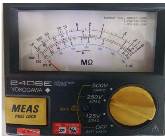
Set the measurement range to 250 V
