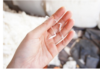
PPP (polypropylene) fibre, an example of contamination which seriously affects the quality of final products
