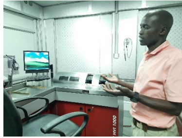
The testing facility at the CDO lab in Kampala. It can test length, uniformity, and strength of the fibre.
