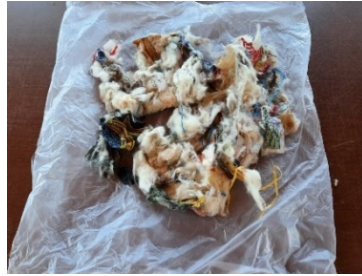
Examples of contamination picked at a spinning mill abroad which received lint cotton from Uganda
