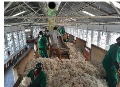
Picking inside the ginnery building, on a belt conveyor
