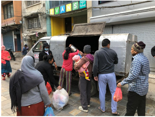
Dump truck with covers before improvement (Mixed waste is loaded through the center opening)
