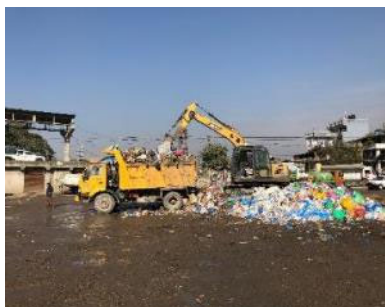
Transshipment to secondary transfer vehicles using a backhoe.
