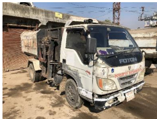
Dump Truck (Bin Carrying Foton)
