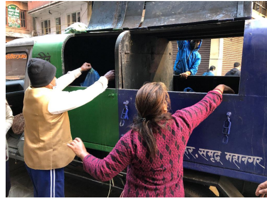
Dump truck with covers after improvement (A partition has been installed in the center, and openings have been created in the front and rear to allow for separation collection)
