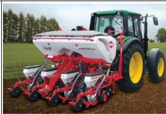
4 row seeder in Japan, seeding width is about 2 m
