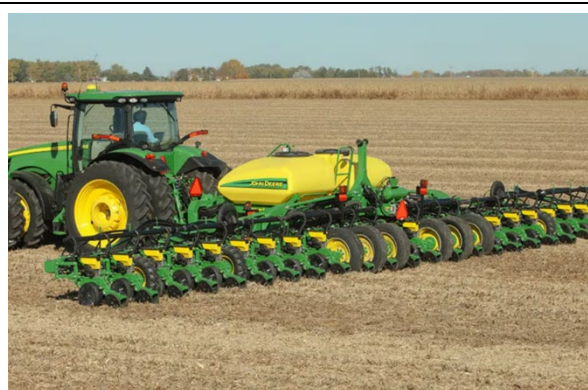
Big seeder connected to a tractor, seeding width is about 10 m
