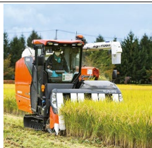
KUBOTA (Japan) Approx. 130 hp, Cutting width 2.4 m, Head-feeding combine harvester
