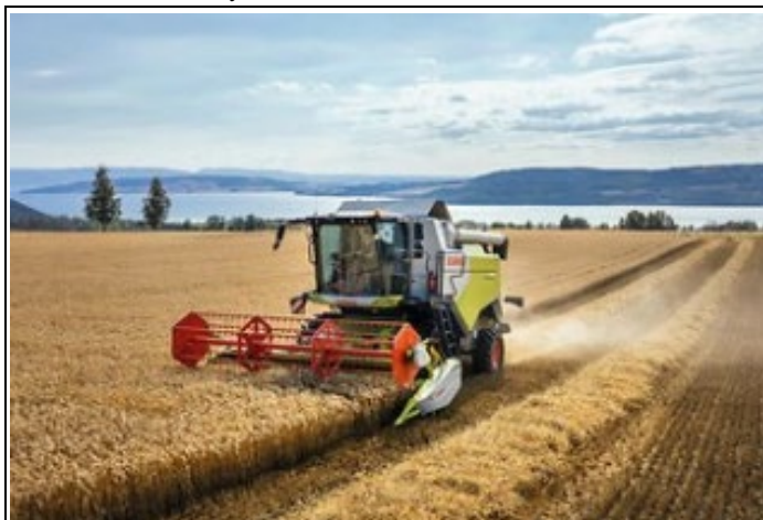
CLAAS (Germany) Approx. 400 hp, Cutting width 5.4 m, Conventional combine harvester
