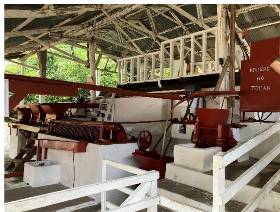
Part of the wet mill. Cherry pulp is removed in multiple steps from the top, then parchment goes to the drying process.
