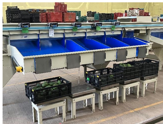
Avocados sorted by size. Brush polishing is done automatically in the lane at the back right, and the fruit is sorted in the front portion.
