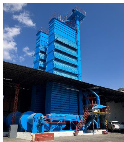
A dryer installed in a rice mill. Since the rice is not dried in the field, it must be dried early and over a long period of time after harvest to ensure that quality is not compromised.
