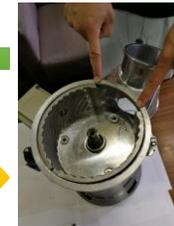
① Put on the milling container and fasten the 3 screws for the container
