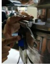
③ Remove the 4 screws from the safety switch
