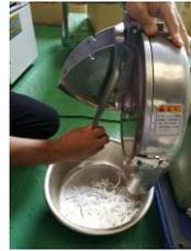
⑦ Push in the onion by the lever (Standard setting: Cut into 3mm)
