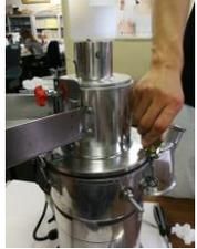
② Remove the upper tray by removing the two screws
