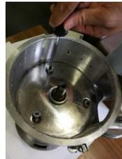
⑤ Remove the milling wall. Turn the outer bolts counterclockwise with a 13mm spanner and a screwdriver to remove.
