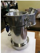
⑥ Remove the 3 screws from the milling container
