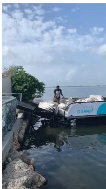
Debris that is removed by the Interceptor™ Tender is transported to an offloading site for sorting and disposal.
