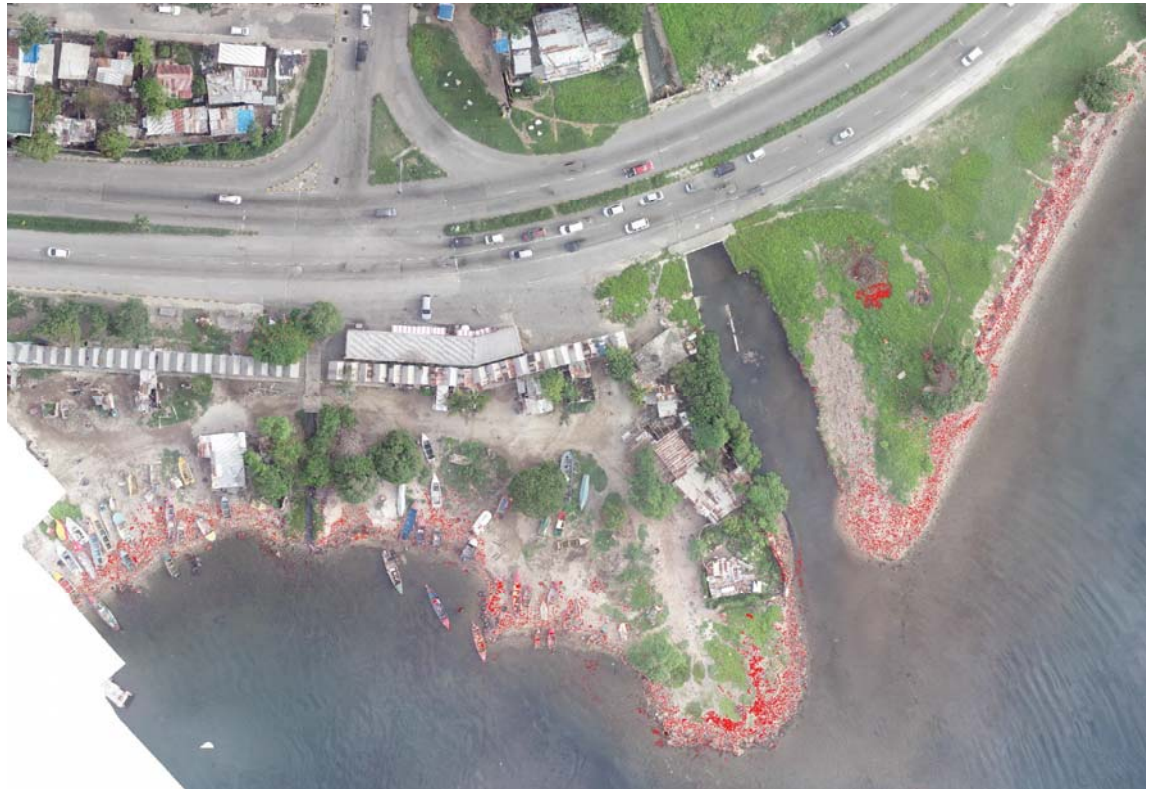
Remote sensing techniques used to classify beached solid waste at Franklyn Town Gully
