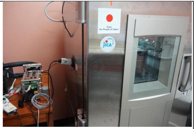
temperature and humidity chamber (right side) Humidity working standard (left side)
