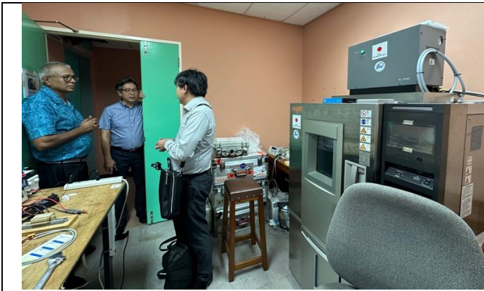
Photo from the back of the calibration laboratory (temperature and humidity chamber on the right side)
