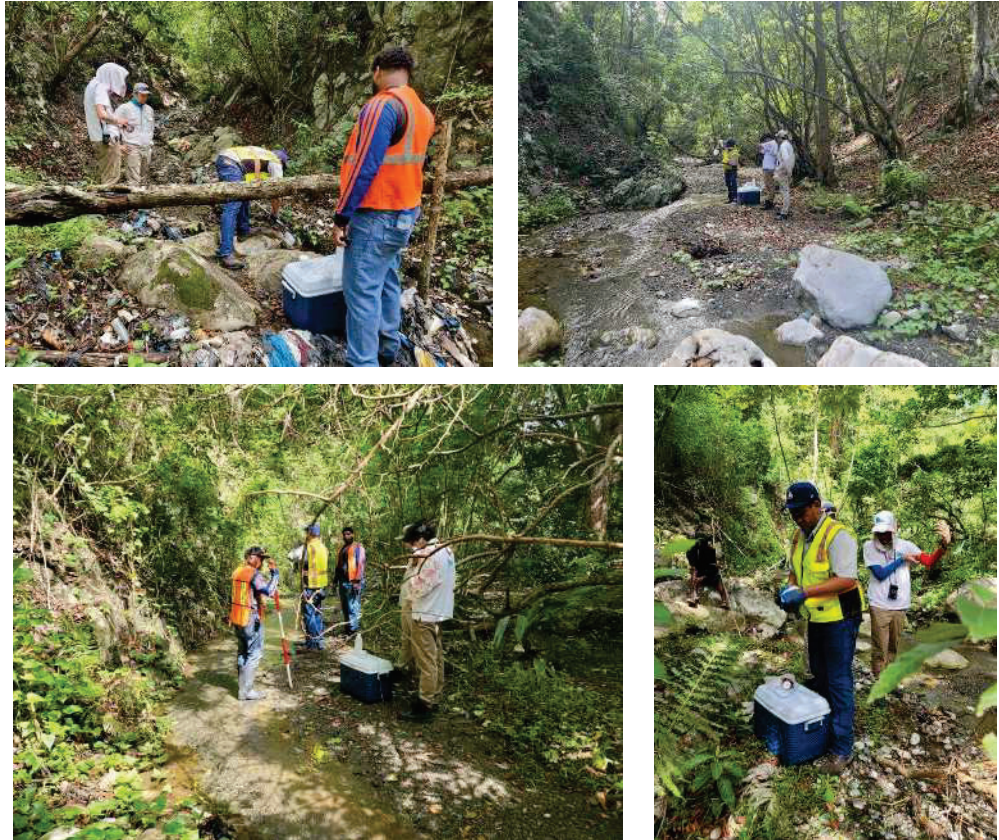
Image 8. Sampling process for water quality analysis
