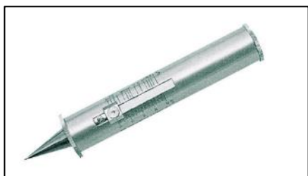
Photo 10. Yamanaka soil Hardness tester
