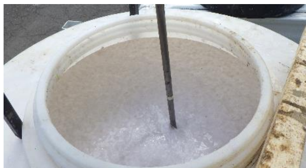
Photo 19. Wood pulp (toilet paper) that has been stirred and turned into sludge
