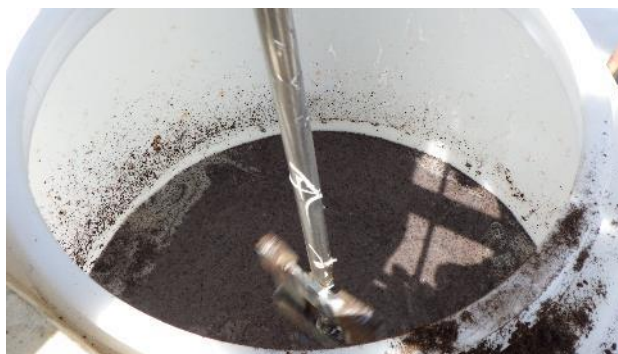
Photo 20. Soil being stirred
