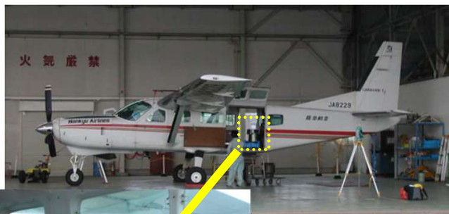
The digital aerial camera mounted on the survey aircraft
