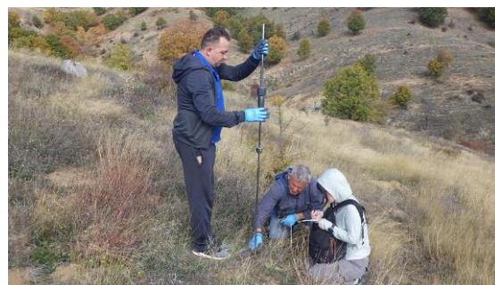
Photo 21: Soil penetration test by Soil penetrometer
