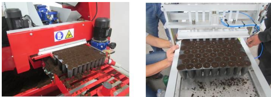
Photo 26: Automatic soil filling machine and sowing machine
