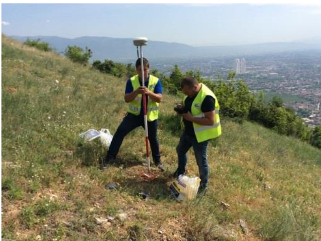
RTK GPS survey conducted in Mt. Vodno
