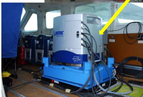
The digital aerial camera mounted on the survey aircraft
