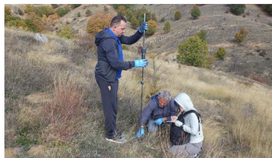
Photo 21: Soil penetration test by Soil penetrometer
