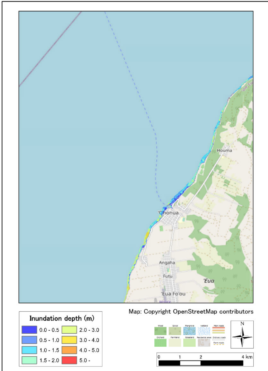
Figure 2.6.140 Max inundation depth distribution (Unnamed1, H=90m)
