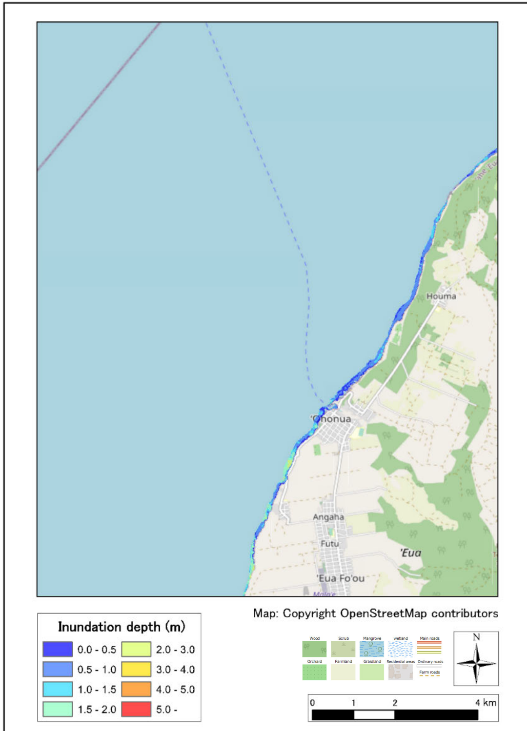
Figure 2.6.132 Max inundation depth distribution (Unnamed1, H=60m)
