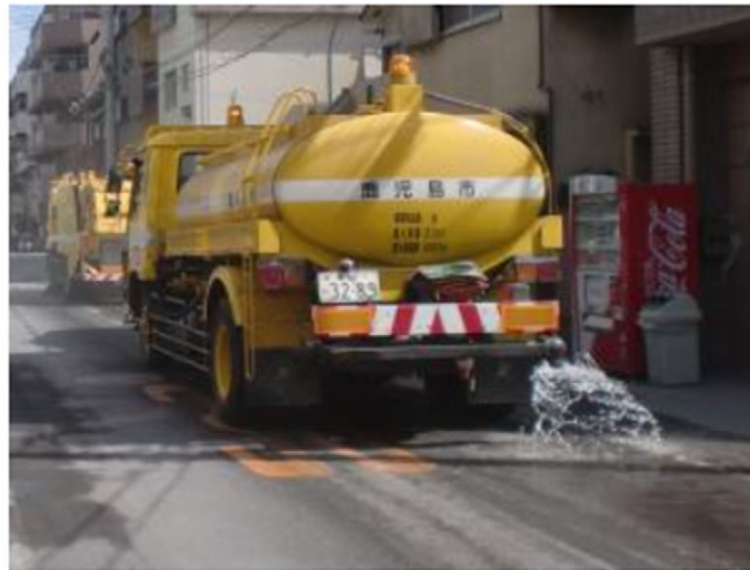
Figure 3.3.8 Water Sprinkler Truck (sprinkling water to prevent volcanic ash dispersion)
