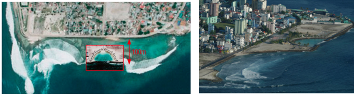
Figure 3.3.2 Before (left) and after (right) installing a tsunami embankment in the Maldives
