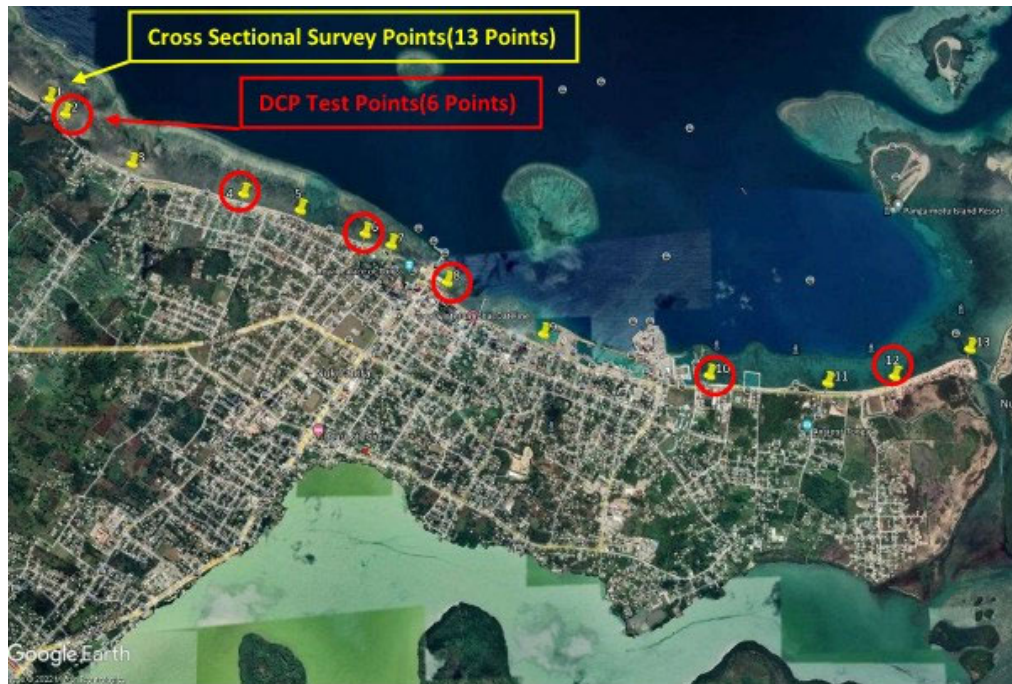
Figure 4.1.8 Location of Cross-Sectional survey and DCP Test at Nuku'alofa
