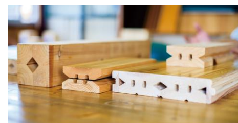
Combining hard-to-use parts to laminated lumber with improved yield
