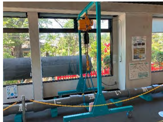
Figure 9-5 [Kubota] Bending experiment equipment of HRDIP
