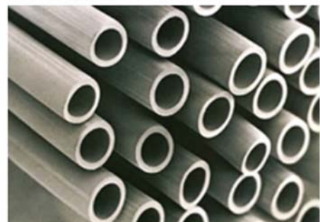
Enlarged cross section of hollow fiber membrane
