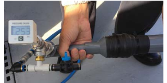
③ Apply tie band to prevent back rush.
