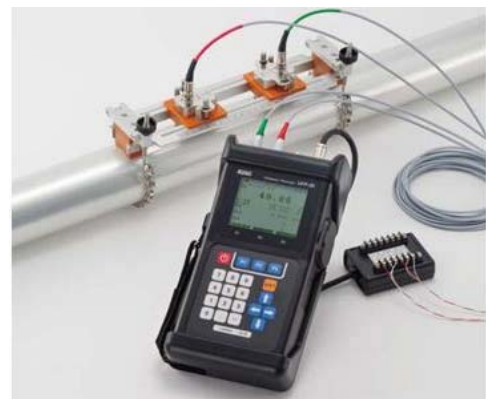
Portable ultrasonic flow meter UFP-20
