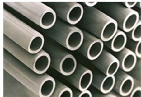
Enlarged cross section of hollow fiber membrane
