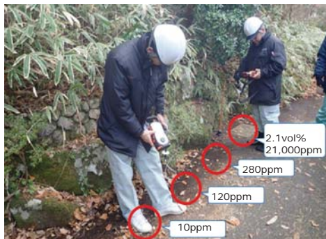
The max. value detected in valve box of fire hydrant
