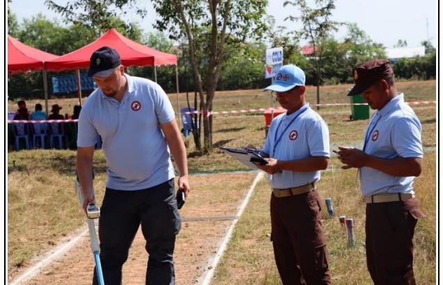
Training participants from Ukraine using ALIS to detect buried objects under the guidance of CMAC3 (TIMA)
