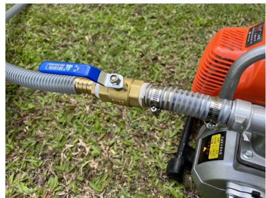
12. Valve connected to engine (if no valve it is okay)
