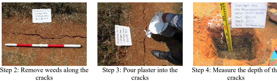
Figure 3.3-2 Procedure of Plaster Survey
