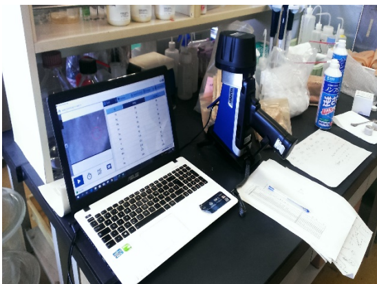
Figure 2: Soil nutrients measurement using the portable XRF
