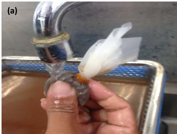
Figure 1: (a) simplified (Nylon mesh) and (b) conventional methods for particle size distribution analysis in Kyoto university lab
