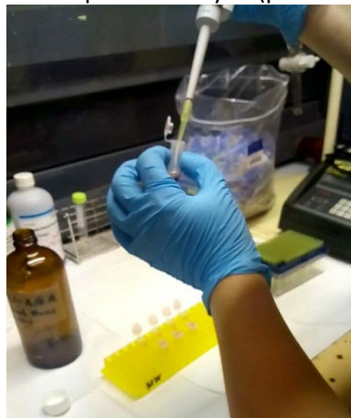
DNA extraction by separating the aqueous phase (photo: Sarah)
