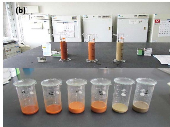
Figure 1: (a) simplified (Nylon mesh) and (b) conventional methods for particle size distribution analysis in Kyoto university lab
