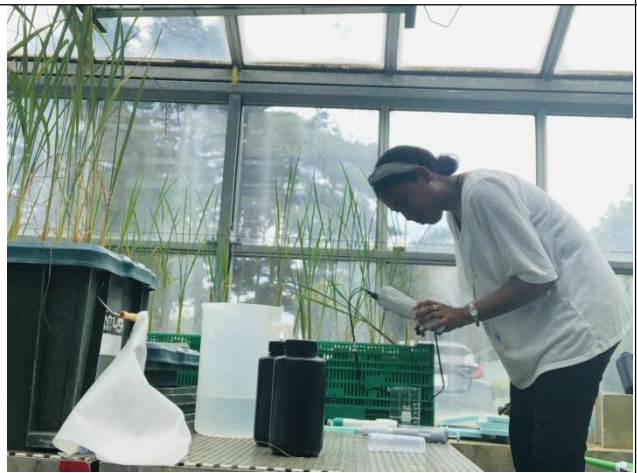
PH measurement of the nutrient solution
