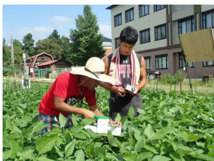
Gas exchange measurement on soybean plant using MIC 100 at Kyoto university
