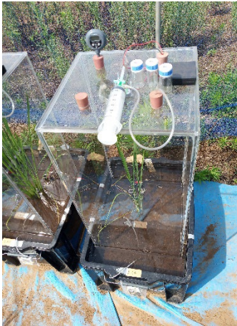
GHG sampling and plant parameters measurements in pot experiment
