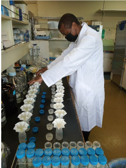
Extraction procedure for P fractionation
