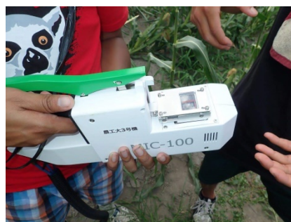
Gas exchange measurement on soybean plant using MIC 100 at Kyoto university
