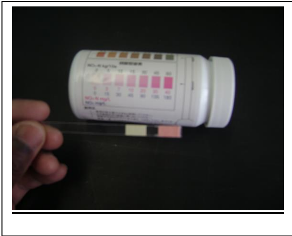
Test rapid for the nitrate at Kyoto University
