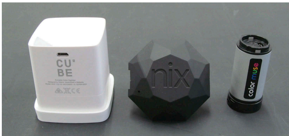
Figure 1. Three types of low-cost colorimeters controllable with a smartphone or tablet. Cube (left), nix pro (middle), and color muse (right).
