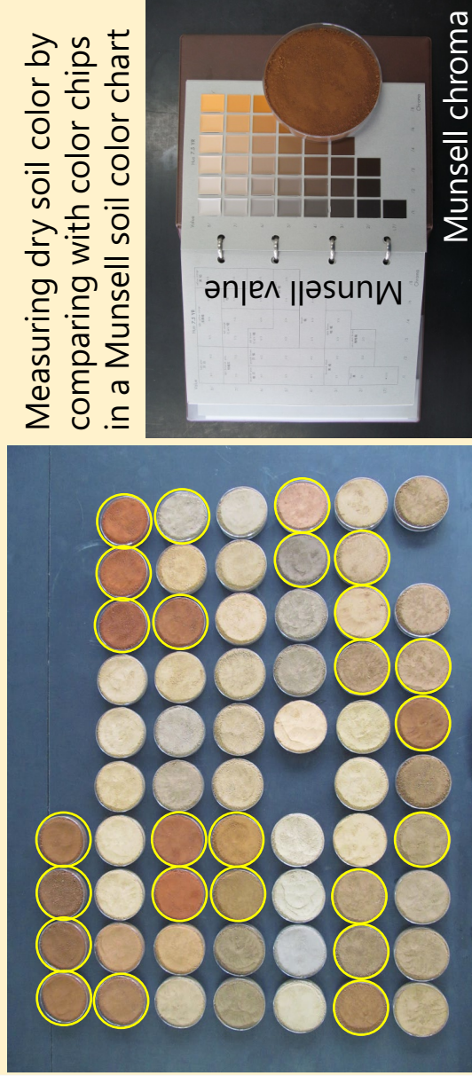
Figure 1. Air-dried, 2-mm sieved soils from rice fields in Madagascar. Yellow flamed samples show upland rice soils.
