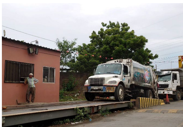
The weight of the transport vehicle is measured at the entrance of the disposal site in Managua City.
