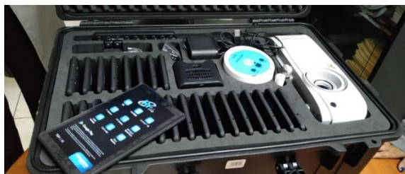
Tomi kit. (Projector, speaker, data sever (round device), tablets (25 devices)
