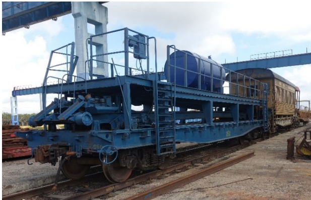
Long rail unloading machine
