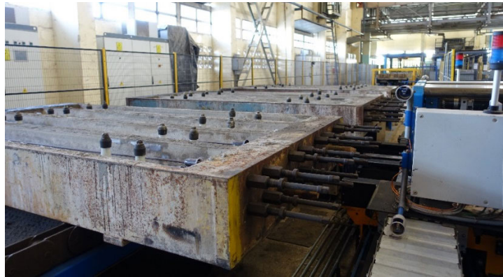
PC sleeper mold with tension bar before concreting
