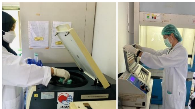
Research with the provided equipment at DOF (Left: tabletop centrifuge, right: nitrogen evaporator)
