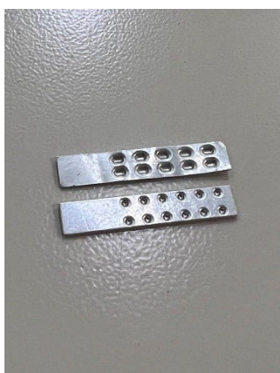
Cryopreservation using aluminum cooling plates (left and middle)
