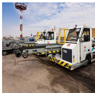
Belt Loader Vehicle (source: JICA)
