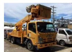
Boom truck with bucket and winch
