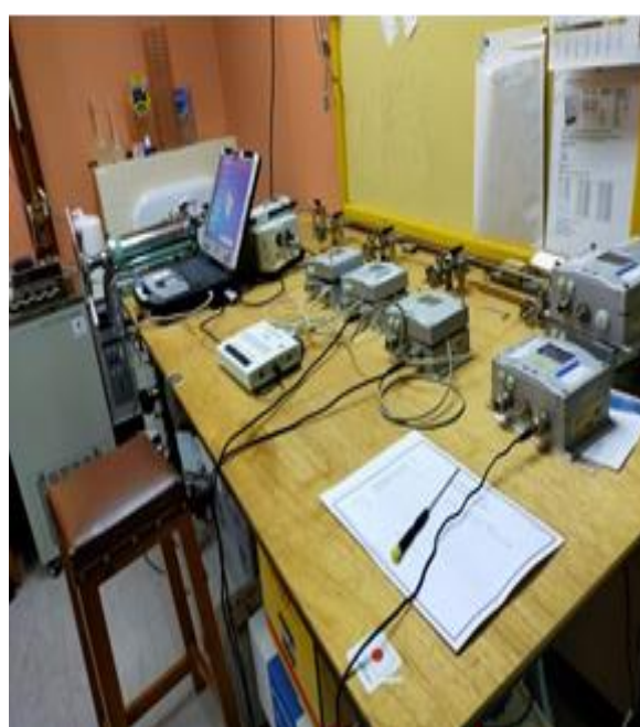
Digital barometer calibration namely (PTB series) JICA provided Tough Book HP laptop and calibration equipment.
