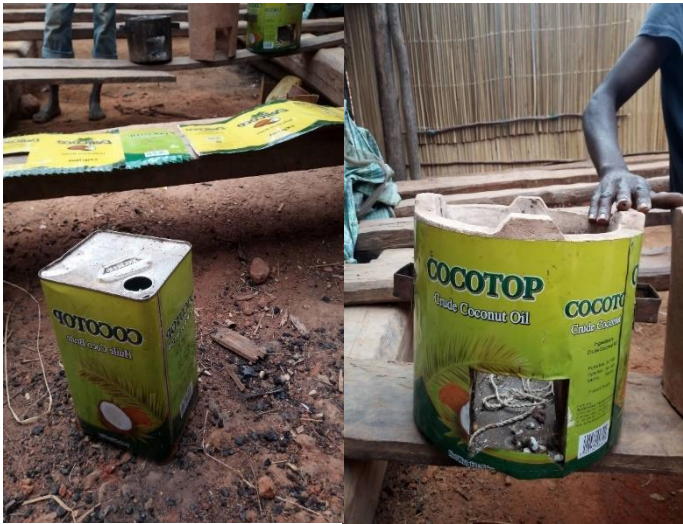
Improved kitchen stove made with recycled materials.
