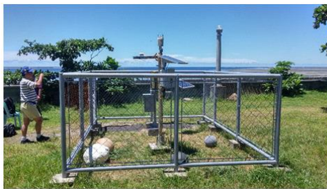
An Automatic Rain Gauge equipment installed for radar calibration and quantitative precipitation estimation
