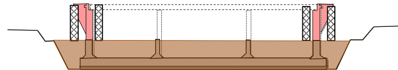
Step-5 Wall Concrete Casting Stage-2.1 (Outer Wall)
