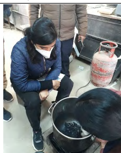
Preparation of bituminous mix by heating and mixing
