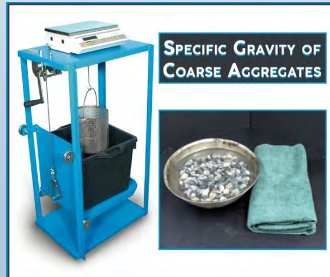
Specific Gravity test; Coarse aggregate
