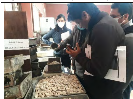
Preparation of aggregate mix (weighing) by participants
