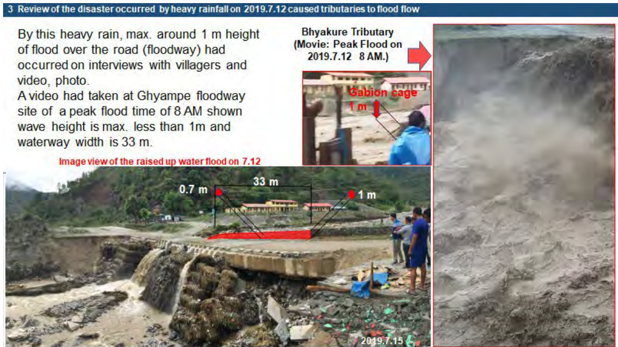
Figure 4-8 Real time video at peak flow Bhyakure on 12 th July 2019
