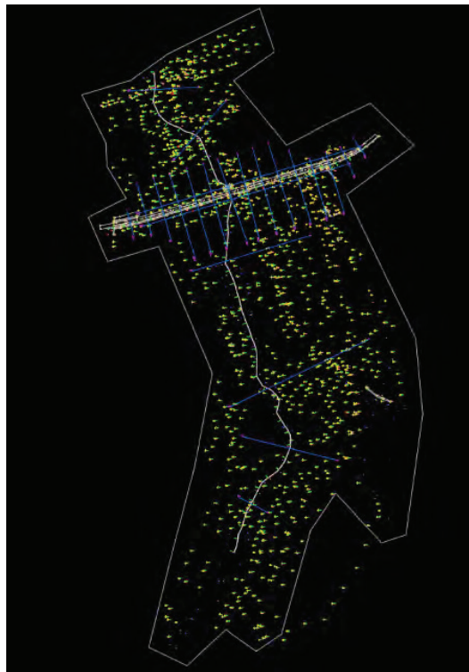
Figure 2: Imported topographic points and setting of alignment of road & stream in Autodesk Civil3D (sample sketch)
