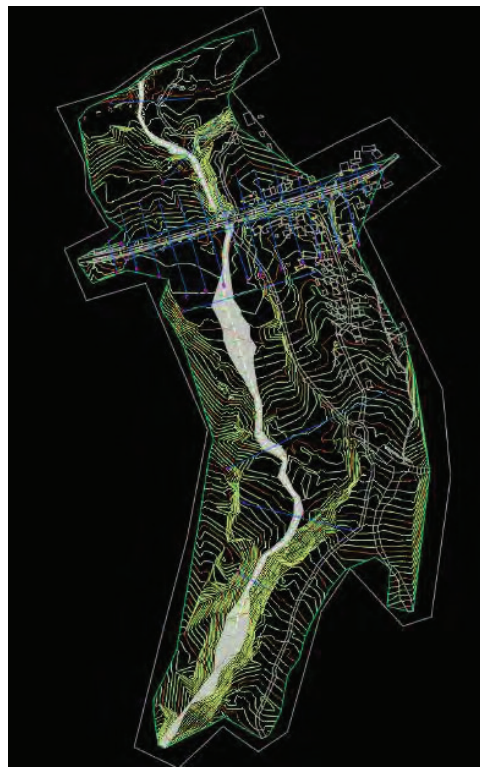
Figure 3: Generated contour lines out of topographic points (sample sketch)
