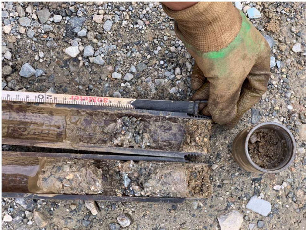
Figure 6: Tube sample at 14 m of borehole B2
