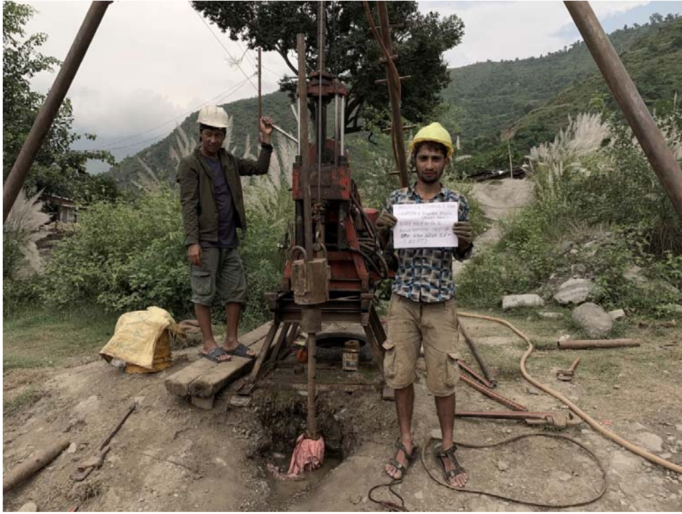
Figure 7: DCPT at borehole G1 (at depth 16 m)
