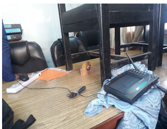
Weather console connect to direct electricity and LAN cable
