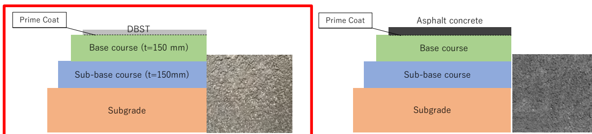
DBST structure applied in the Sindhuli Road
