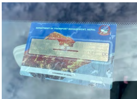
Figure 2.3.2 RFID tag on the windscreen of a vehicle
