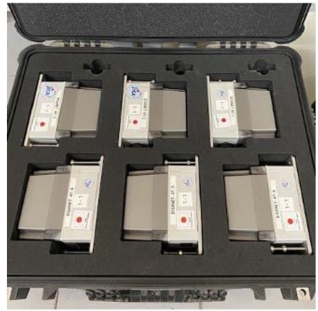
Portable microtremors observation system being used for research at IIITH
