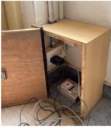
Strong motion sensor (ITK sensor) installed in the IIITH building to conduct constant monitoring
