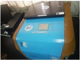
Automated analyzer for screening cells (EasyCyte 5HT)
