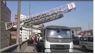
Photo 1. The bridge inspection vehicle in operation at the site (inspection of bridge)
