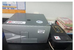
Microplate reader (Infinite 200 pro)
