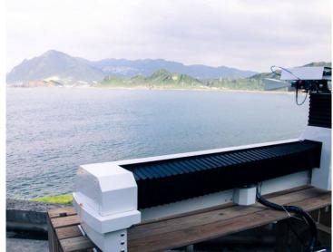
Photo 2 (provided by MMU): MMU utilized the SAR subsystem for further development of a ground-based SAR (GBSAR) to detect land deformation. According to MMU,GBSAR has higher detection accuracy compared to CP/SAR and can detect sub-mm movement on natural or synthetic objects.
