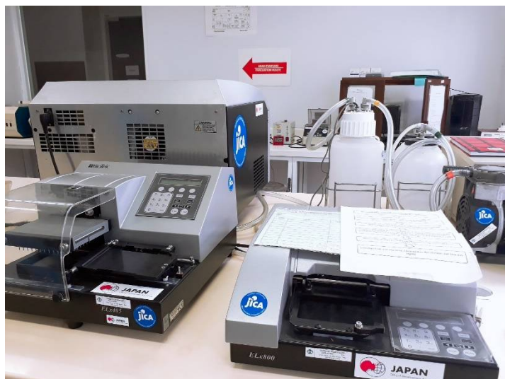
Elisa reader equipment for reading the antigen – antibody bond (University of Indonesia)
