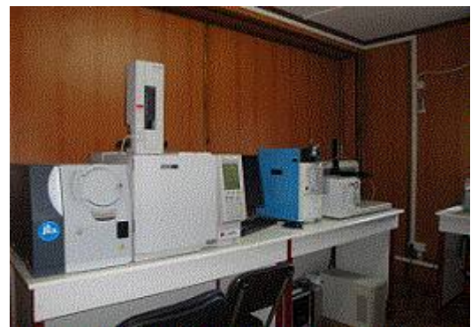
Laboratory equipment (Gas Chromatography/Mass Spectrometry, source: CRL)
